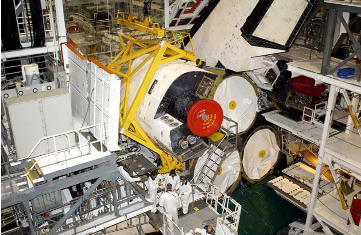
Figure 1-1 - A left APS pod is being removed from the space shuttle orbiter Atlantis.
