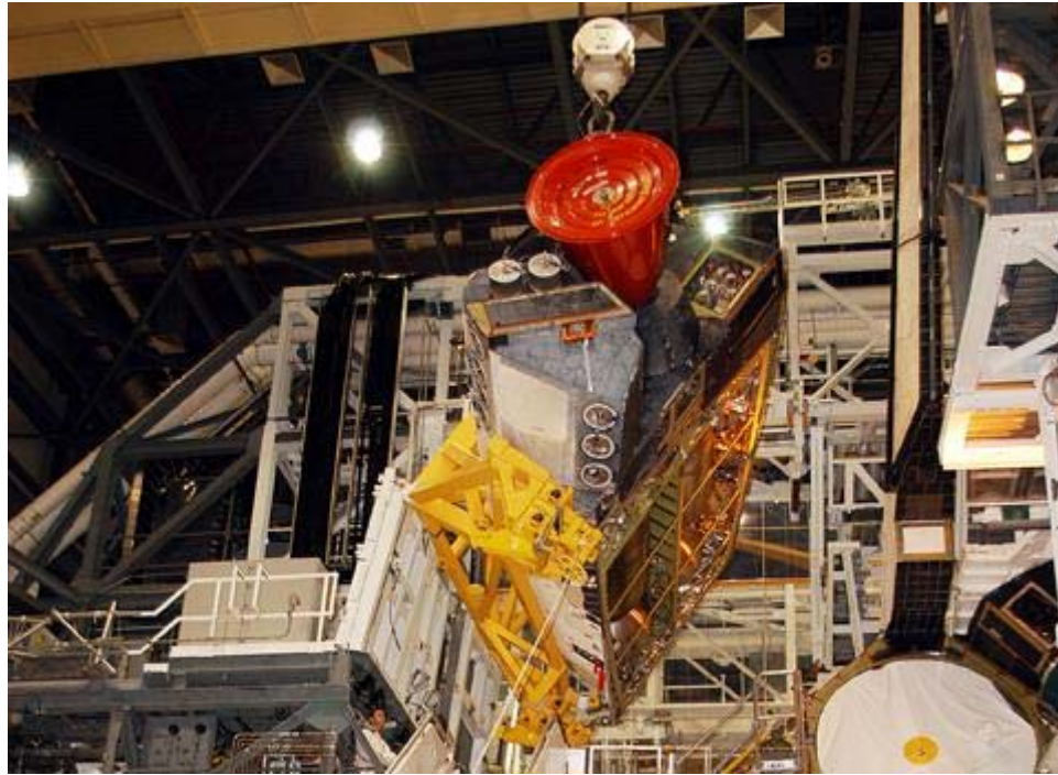
Figure 1-6 - A left APS pod is transported by crane to Atlantis for installation.
