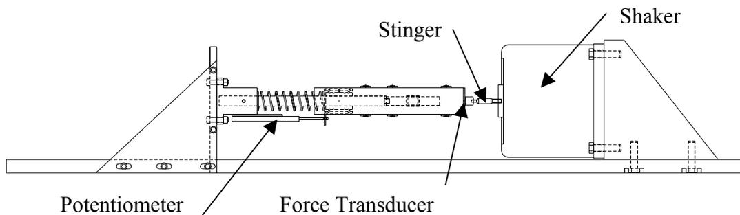
*Figure 3 Friction Damper with Shaker and Transducers (Side View)*
