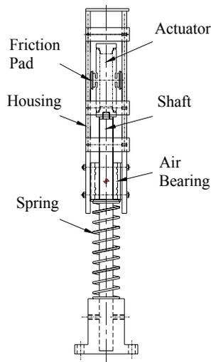
*Figure 2 Friction Damper (Front View)*
