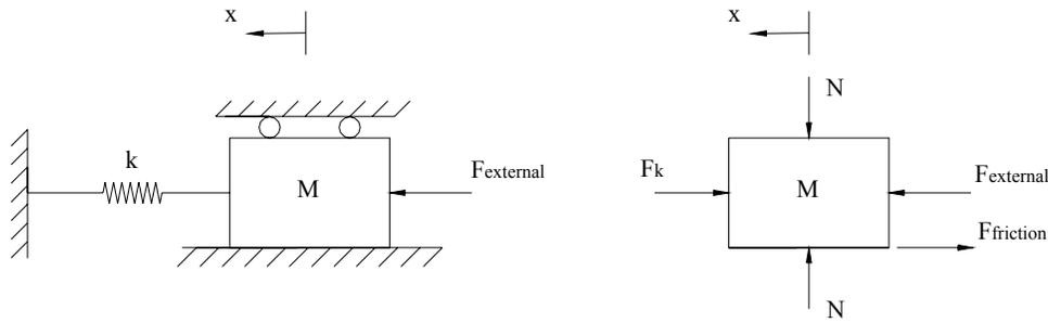
Figure 1 Schematic Drawing and Free Body Diagram
