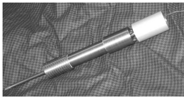
Fig. 9. Double-shaft MR damper made from low-carbon steel
