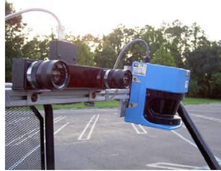
Figure 4.4: Videre Design STH-MD1-C and the SICK ladar
