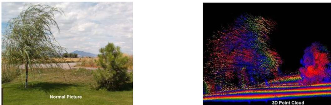
Figure 4.1 Output from the spinning Ladar
