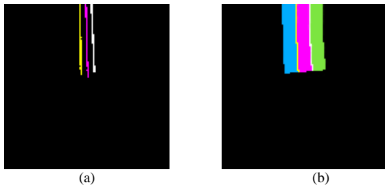
Figure 11. Traversability Grid. (a) With interpolation and estimated lane center line elements. (b) With painted lanes and boundaries.
