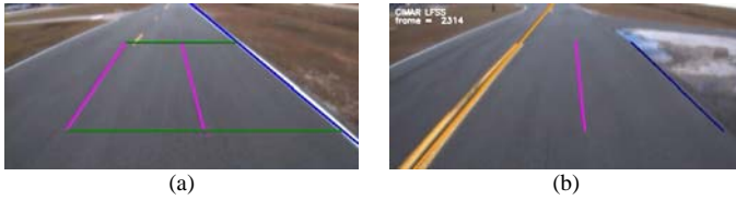
Figure 10. Lane Estimation (a) yellow lane marker (b) white lane marker
