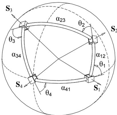
Figure 11: Spherical Four-Bar Mechanism
