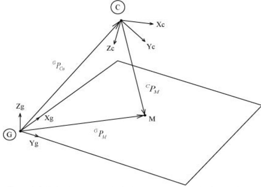
Figure 2: Relation between a point in the camera and global reference frames
