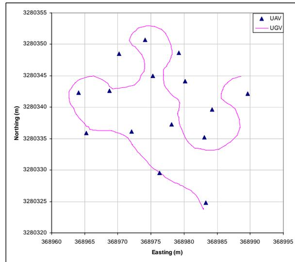
Figure 7: UAV waypoints vs. UGV path
