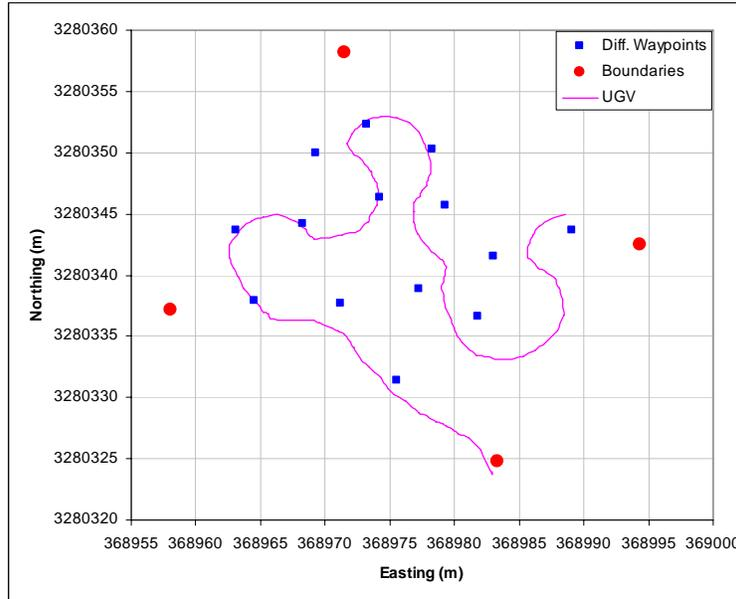
Figure 5: A comparison of the UGV's path to the differential waypoints
