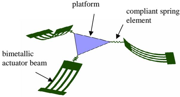
Fig 2. Compliant Microplatform
